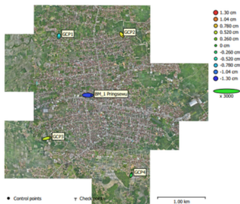
Fig. 4. GCP locations and error estimates. Z error is represented by ellipse color. X,Y errors are represented by ellipse shape. Estimated GCP locations are marked with a dot or crossing.
